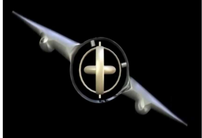
90. Plane tilted, gyroscope compensates
